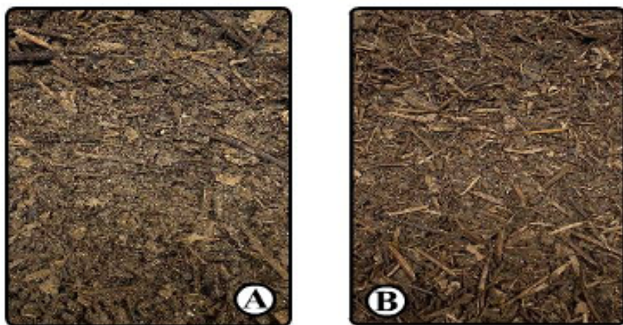
Figure 2. Physical appearance of matured and sieved kitchen waste BA-compost (A) and control without biomass ash (B).
